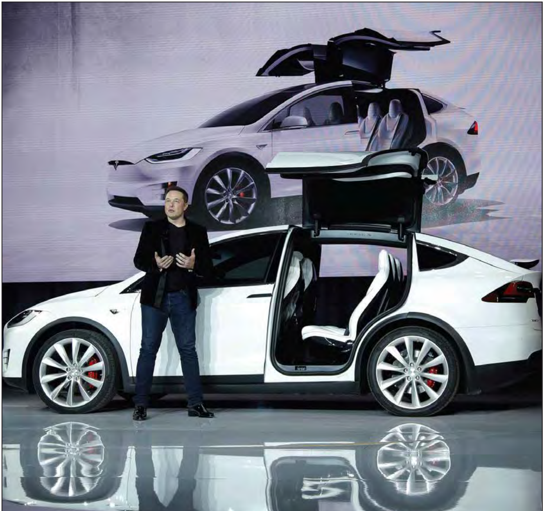
Elon Musk, CEO of Tesla Motors Inc., introduces the Model X car at the company's headquarters. Musk said the Model X sets a new bar for automotive engineering, with unique features like rear falcon-wing doors, which open upward, and a driver's door that opens on approach and closes itself when the driver is inside. (AP Photo/Marcio Jose Sanchez)
